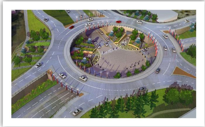
This two-year roundabout study was recently completed, and the findings show an improvement in traffic movement while at the same time demonstrating a dramatic reduction in crashes at this key intersection from its previous traditional 4-way signalized design into a roundabout design. At the 14th & Superior roundabout, injury crashes are down 75%. Those are dramatic reductions and demonstrate how roundabouts protect motorists and save dollars.
